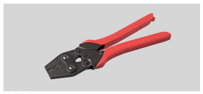
**Crimping tool HWZ 6**Crimping tool for noninsulated terminals from  $0,5\ up\ to\ 16mm^2.$  The ratchet guarantees a permanent high quality crimping result.
