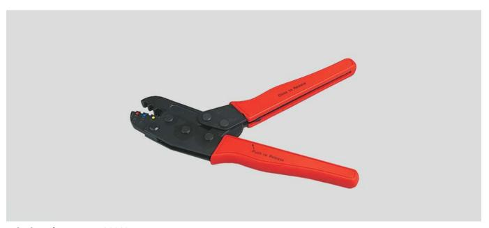
**Jointing clamp type 802/0**For insulated cable lug, with positive lock. Clamping range 0.5 to 6.0mm².
