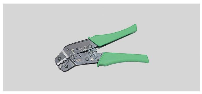
**Jointing clamp type DEB 0560** For insulated and non-insulated core end sleeves, for completely safe clamping with positive lock. Clamping range 0.5 to 6.0mm².
